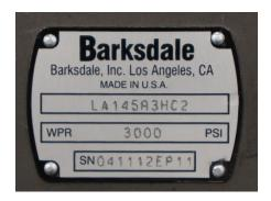
Nameplate is permanently secured to side of valve with the followings information: model part number, working pressure (WPR) and serial number (SN). The first 6 digit numbers of the serial number represent the date of manufacture (XX month/YY date/ ZZ year).
