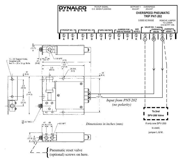
**SPV-200** Solenoid Shutdown Valve (showing input from PNT-202)
