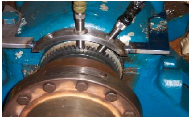
Figure#3: Pickup mounting example (Pickup probe is collinear with radius of the gear)
