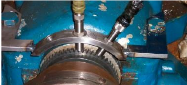
Figure3: Pickup mounting example (Pickup probe is collinear with radius of the gear)
