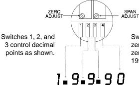
Switch 4 adds a dummy zero (fifth digit, fixed zero) to extend range 1999 to 19990.
