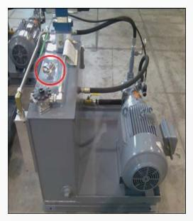
At the core of every hydraulic power unit (HPU) is the reservoir, which holds the hydraulic fluid. Controlling fluid level and temperature in the reservoir is critical to efficient operation. Elevated temperatures can result in fluid degradation, loss of lubrication and destroyed seals. Low fluid level can contribute to damaged pumps and cavitation – a condition that erodes metal surfaces within the system and negatively impacts performance.
