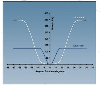
Barksdale's patented proportional air flow design optimizes air usage within the vehicle air suspension system. The Barksdale height control valve reacts instantly to large suspension movement, providing maximum rated flow to rapidly restore vehicle ride height. Smaller changes in ride height result in proportional reductions in the volume of air flow to or from the air springs. Air is conserved and ride height overshoot and undershoot are virtually eliminated.
